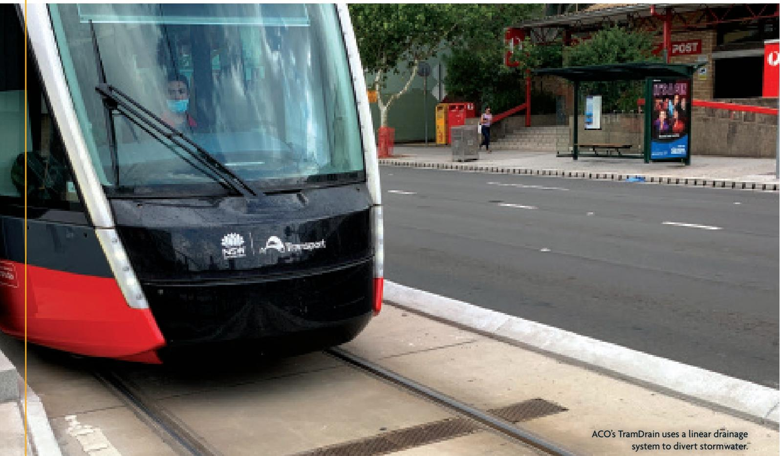
ACO's TramDrain uses a linear drainage system to divert stormwater.
