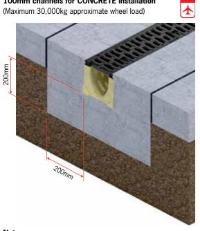
Poor site conditions and low load bearing pavements will require an increase in the dimensions shown in the illustrations to meet both the vertical and lateral loads. It is the customer's responsibility to ensure that the complete design and construction of the encasement is suitable for the application. If in doubt, seek engineering advice.
