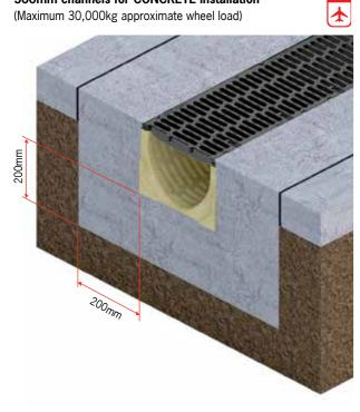
Note: 1. Grate should be 3mm below pavement surface.
