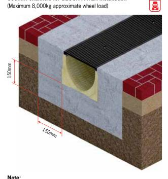
1. Grate should be 3mm below pavement surface.
