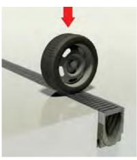
Static loads are the weight applied vertically onto a trench drain with no other movement. Static loads are used in load testing a grate or trench drain, as they provide an objective measure to rate products. They are not typically found in real-life scenarios.
