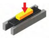
Diagram shows test block positioned centrally on grate.
