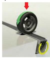
Forces created by dynamic or moving loads tend to twist trench drains and grates out of position. The more movement the greater the dynamic load. Forces also rise rapidly as the traffic speed increases.
