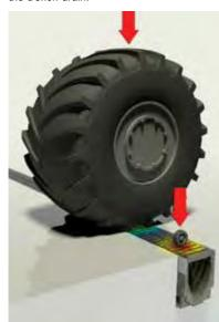
Small tyres and solid tyres concentrate load onto a small contact area, which exerts a higher stress. This application requires a drainage system with a higher load rating.
